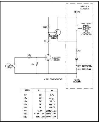
Figure 4-8. External Trigger Circuit
